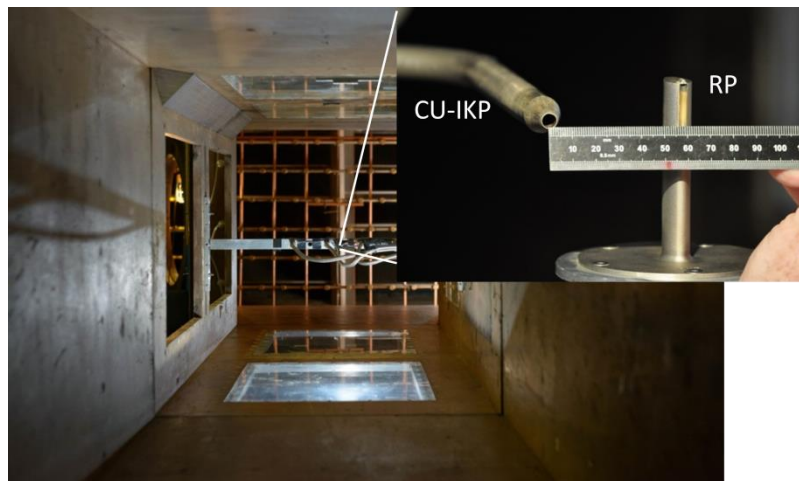
Figure 10: Instrumentation layout in CU tunnel test section and separation distance between RP and CU-IKP.
