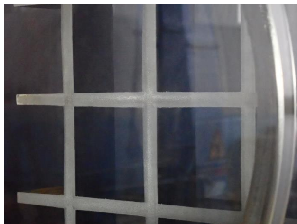
Figure 6: Accretion grid used for MW probe evaluation at MinDef
