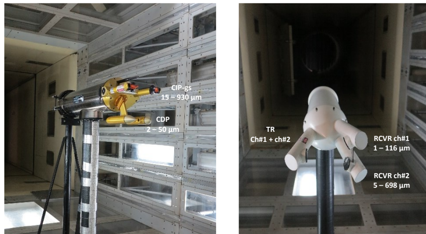
Figure 8: DLR CCP (Cloud Combination Probe) on the left, installed in the centerline of the CIRA IWT test section during the PSD/MVD measurement slot. CIRA 4D-PDI on the right installed with sample volume located on the centerline, in the same position of DLR CCP.
