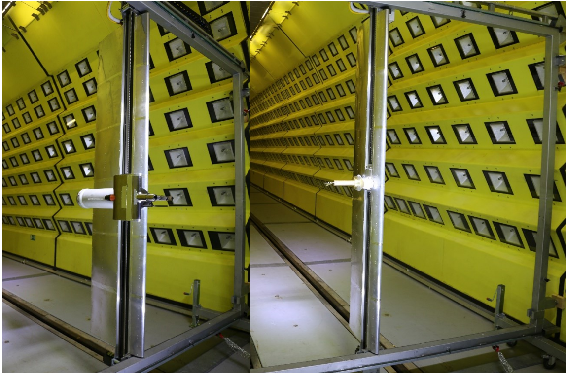
Figure 8: PSD (left) and LWC instrumentation (right) mounted on a traversing system in the RTA IWT
