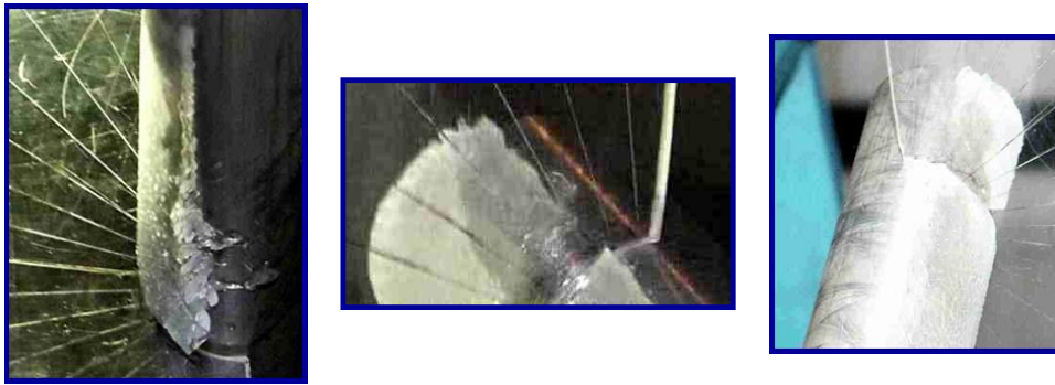
Figure 33: Change of ice buildup forms on three cylinders
