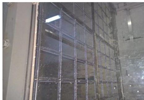
Figure 25: The measurement grid in the AHT SD working chamber during cloud uniformity calibration
