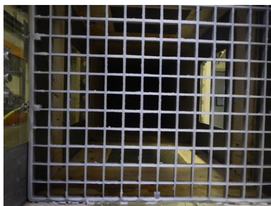
Figure 36: Ice uniformity measurements using an icing grid in the full test section of the AIWT
