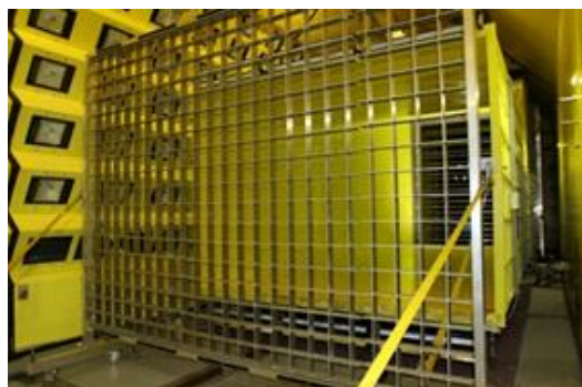
Figure 21: Photograph of the ice accretion grid installed at the RTA IWT
