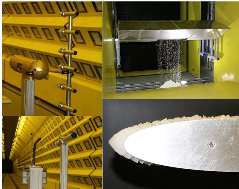
Figure 10 IAG SnowFall snow generation system into RTA Climatic Wind Tunnel and calibration
