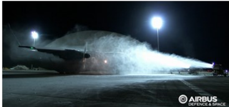
Figure 2 A400M snow tests with a snow gun; credit: Airbus Defence & Space
