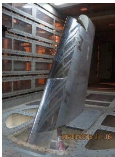
Figure 5 The business jet 3D wing tested in Appendices C & O in CIRA IWT
