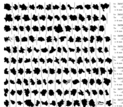
Figure 2: Representative snowflakes with sizes around 2 to 3 mm, obtained in flight test at -3°C (Source: Airbus)
