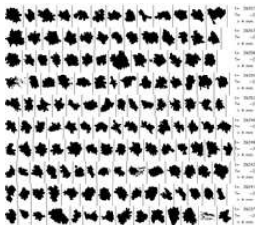
Figure 14: Representative snowflakes with sizes around 2 to 3 mm, obtained in flight test at -3°C (Source: Airbus Helicopters)
