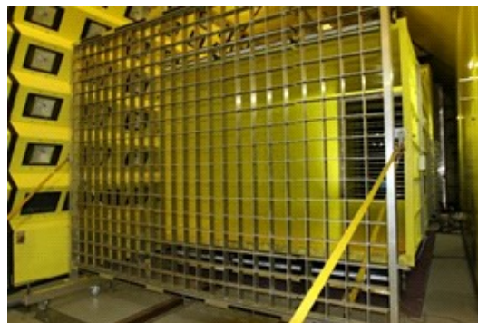
Figure 9: Photograph of the ice accretion grid installed at the RTA IWT
