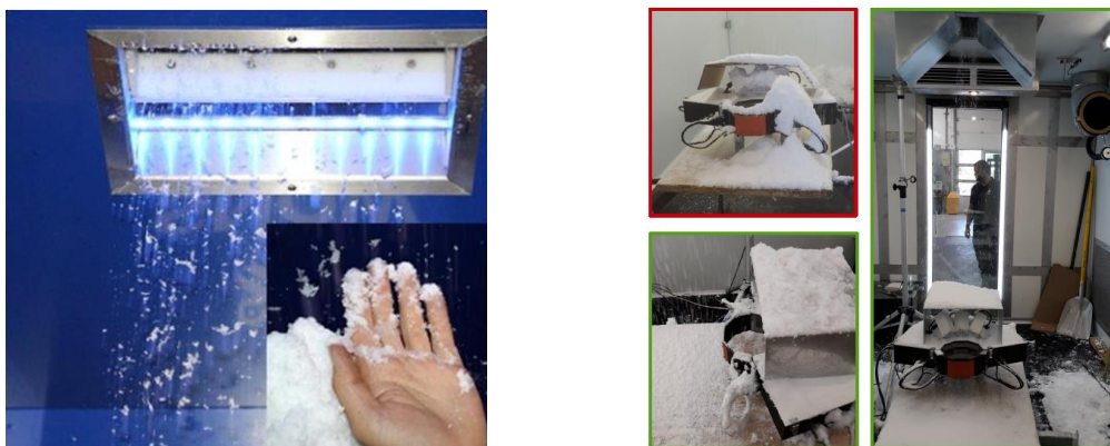
Figure 5 – IAG rotating cylinder for snow production (left) and climatic chamber test setup with MASC instrument for characterization of the artificial snow particles
