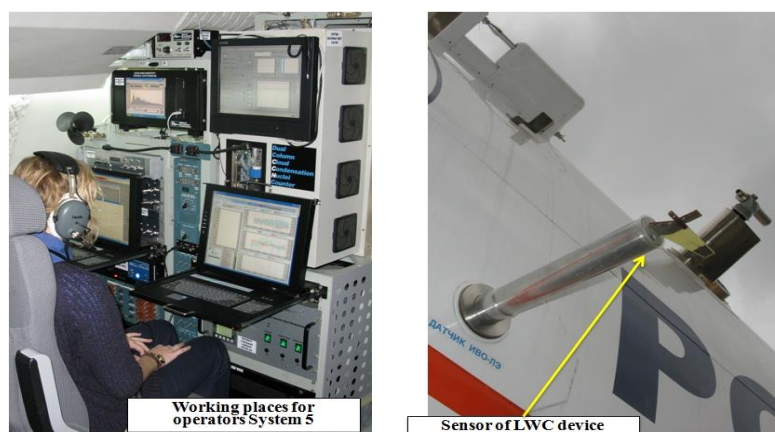
Figure 13 - Sensor for liquid water content (right). Working places for on-board operators (left)
