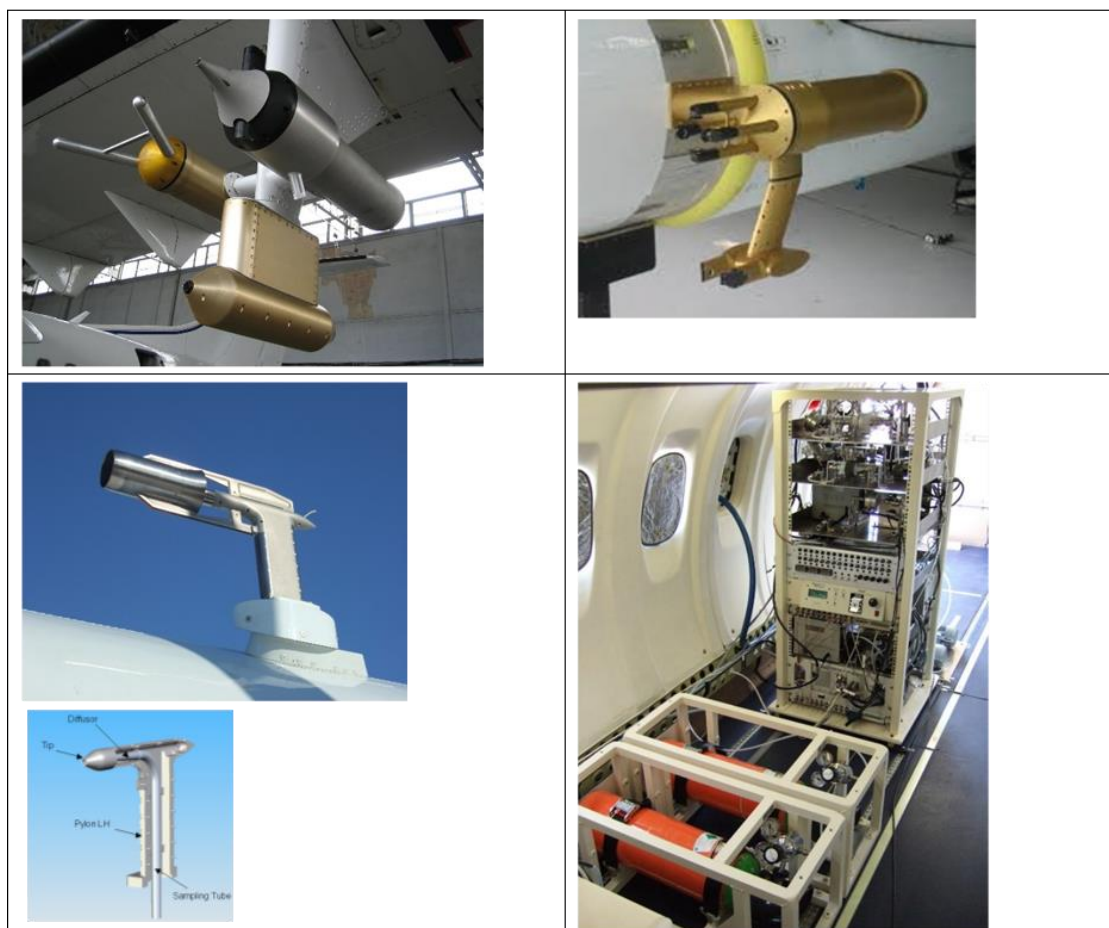
Figure 17 – ATR-42 in situ instrumentation: Polar Nephelometer, CPI, PIP dummy (upper left), 2D-S / FCDP (upper right), CVI cloud inlet (lower left) and measurement rack, synthetic dry air for CVI (lower right).
