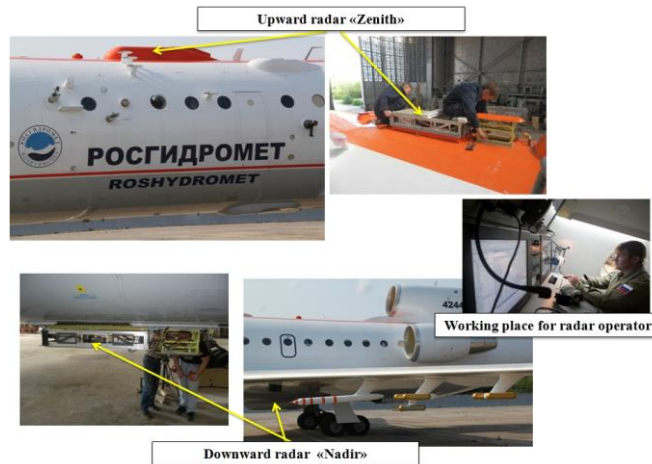
Figure 14 - Outside radar antenna of radars and working place of on-board operator
